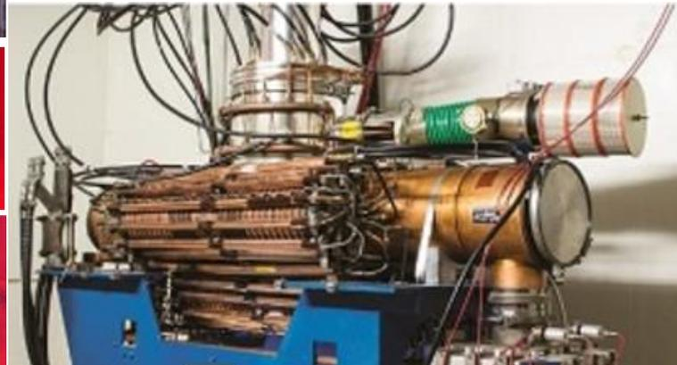
CW 50.6 MHz cavity of PSI cyclotron.  $V = 1.2$  MV
