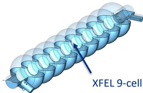
XFEL 9-cell 1.3 GHz SW cavity
